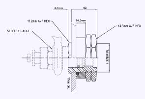
The tank boss is only suitable for use with tanks of wall thickness from 1.58mm (1/16") to 7.9mm (5/16") hole diameter of 42.0mm is required in the tank wall.
