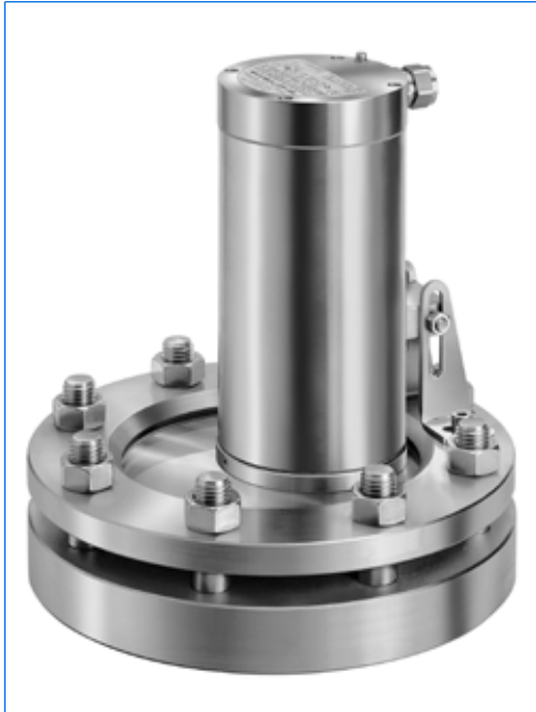
Sightglass light fitting type EdelEx 50 dH Sch K2, 50 W, 230 V, Ex d IIC T4 Gb, Ex t IIIC T130°C Db IP67, Ex II 2 G + D, mounted on circular sightglass to DIN 28120, PN 10, DN 150.
