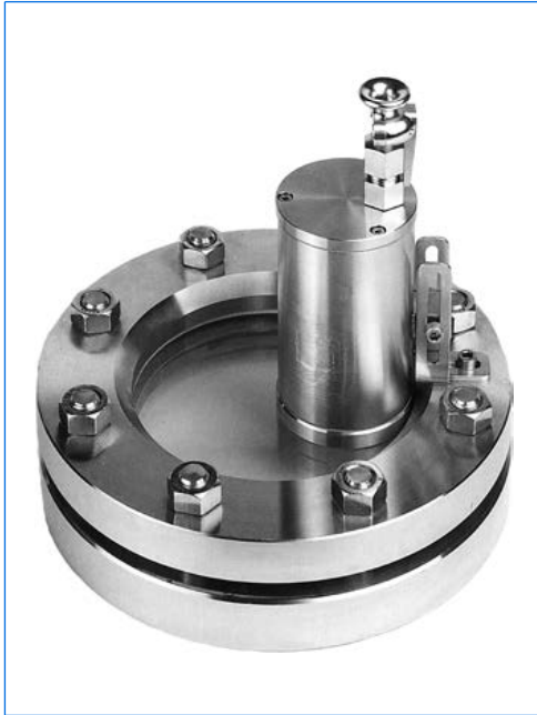
Sightglass light fitting type EdelEx d PowerLED Sch K1, 7 W, 24 V AC/DC, Ex d op is IIC T6 Gb, Ex tb IIIC T80°C, IP 65/67, Ex II 2 G + D, mounted onto circular sightglass to DIN 28120, PN 10, DN 125.
