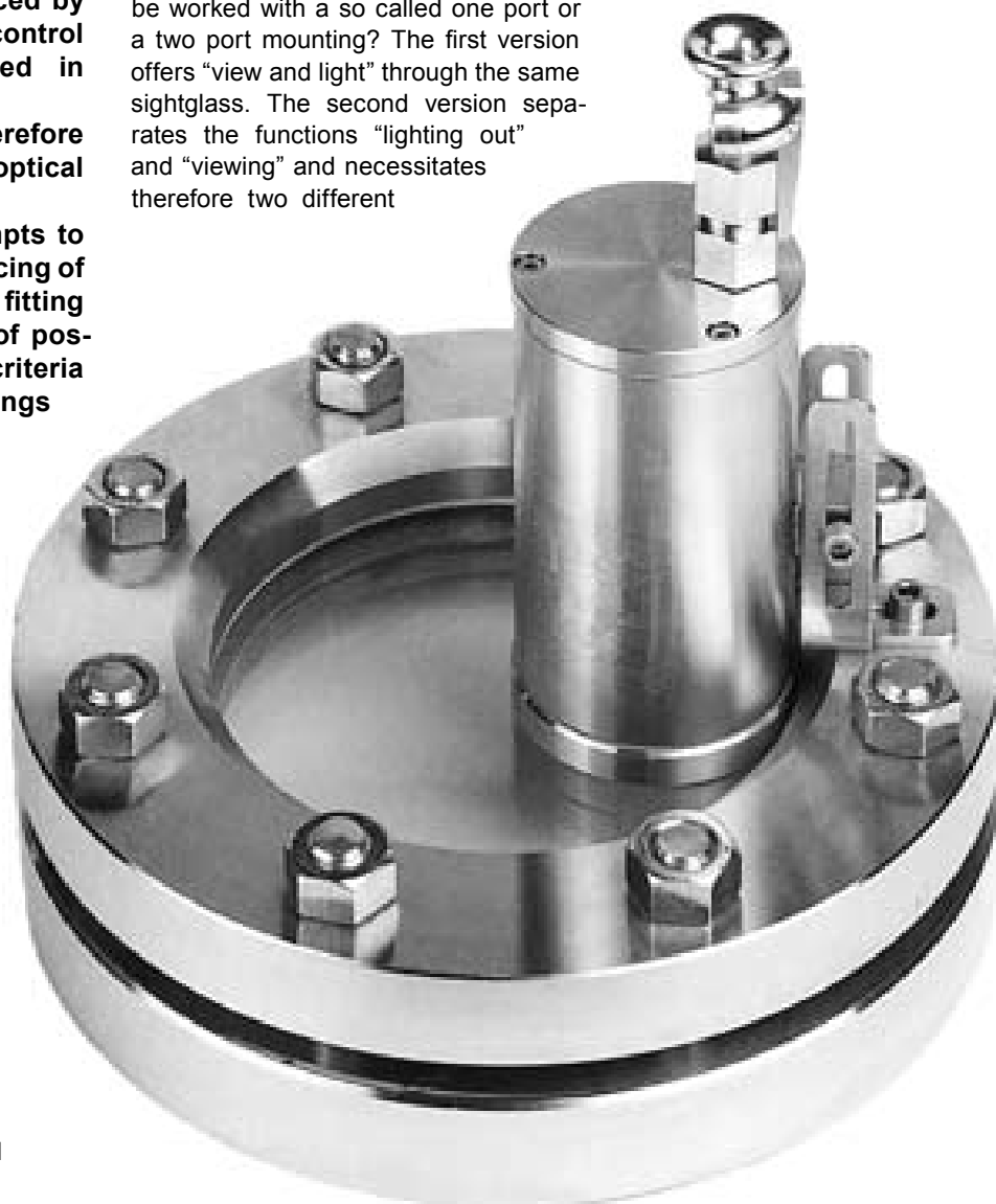
Fig.1 EdelLUX® light fitting type EdelEx, completely in stainless steel, 20 W, 24 V, Ex d IIC T4 Gb, Ex t IIIC T130°C Db IP67, mounted on a VETROLUX® sightglass to DIN 28120
