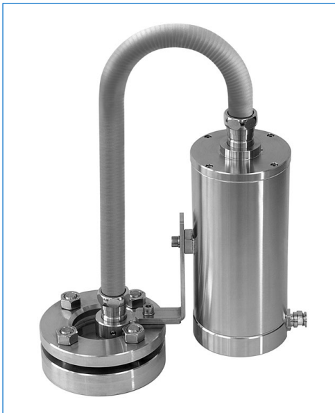
Stainless steel fibre-optic lightpipe light fitting, type fibroLUX E 5035 W W2 sp, Ex d IIC T4 Gb, Ex t IIIC T130°C Db IP67, Ex II 2 G + D, 35 W, 24 V AC, fixation of the light source by bracket "W", fixation of the lightpipe by universal support "W2" onto sightglass to DIN 28120, DN 40, PN 10
