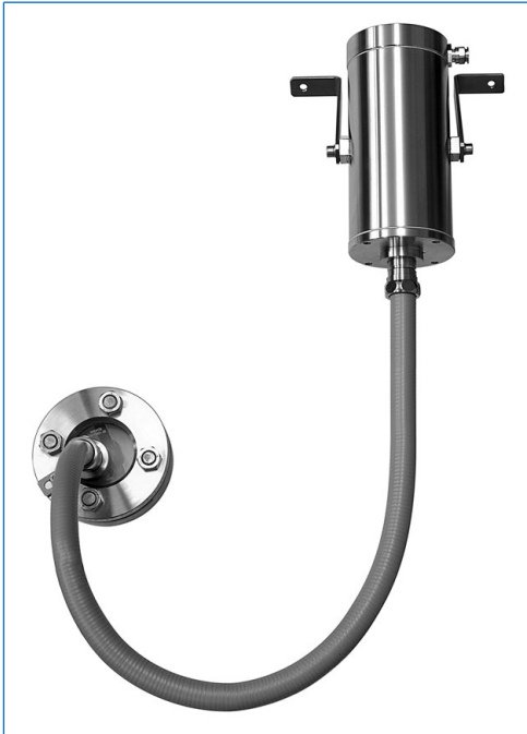
Stainless steel fibre-optic lightpipe light fitting for use in hazardous areas, type fibroLUX E 5035 X1 W2, Ex d IIC T4 Gb, Ex t IIIC T130°C Db IP67, Ex II 2 G + D, 35 W, 230 V, fixation of the light source by fixation legs "X1", fixation of the lightpipe by universal support "W2" onto sightglass to DIN 28120, DN 40, PN 10
