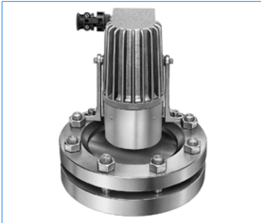
Type PEL 50 deH X2 B, 230 V, 50 W, Ex d e IIC T4 Gb, Ex t IIC T130°C Db IP67, Ex II 2 G + D, with anti-dazzle shield "B", on circular sightglass to DIN 28120, DN 150, PN 10, in version "view and light trough one assembly"
