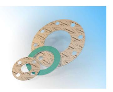
Optimised combination of synthetic fibres and glass-fibre bound with NBR. Premium quality jointing with high temperature resistance in steam and water as well as excellent resistance to oils and hydrocarbons.
