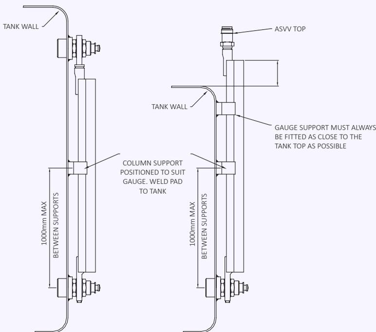
Gauges that have a centre distance greater than 1000mm and open circuit gauges, will be supplied with a column support, so that the gauge can be fixed to the tank wall. The maximum distance between the gauge fixings and a column support or between two column supports should be 1000mm, in the case of open circuit gauges the top most column support should be fitted as close to the tank top as possible.
