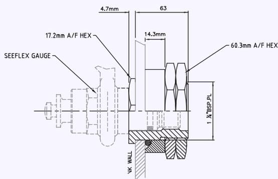
The tank boss is only suitable for use with tanks of wall thickness from 1.58mm (1/16") to 7.9mm (5/16") hole diameter of 42.0mm is required in the tank wall.
