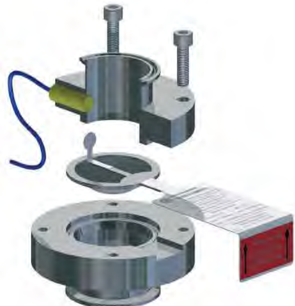
Reverse buckling bursting disc with transmitter with inductive proximity switch in bursting disc holder Type BHS
